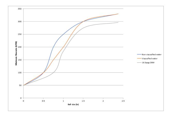
When using 4  $\frac{3}{4}$ " valves the ID of the valve is 1.313" giving a maximum ball passthrough diameter of 1.25". A chart of minimum flowrate required for balls to pass through 4  $\frac{3}{4}$ " tools with non viscosified water is given below.
