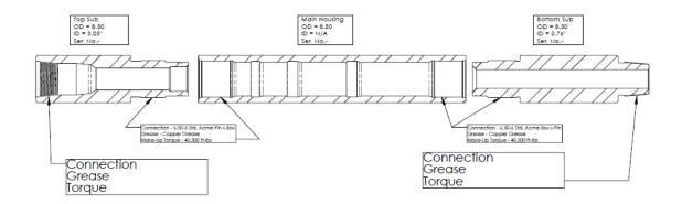
The 7" tool service connections have a 5.5" Standard Acme thread and single o-ring seals. They will normally be torqued to 60% shoulder yield unless otherwise requested.
