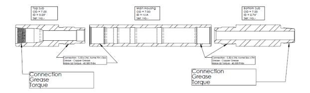
The 4  $\frac{34}{7}$  tool service connections have a 3.5" 8 TPI Stub S=Acme thread and single o-ring seals. They will normally be torqued to 50% shoulder yield unless otherwise requested.
